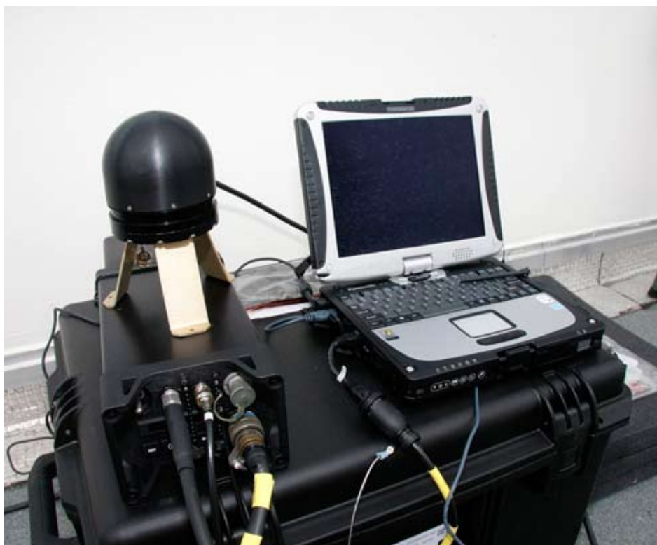
ROVER 4 (Remotely Operated Video Enhanced Receiver) Receiver Antenna and Laptop. [ Source: Metternich/Luftwaffe ]
