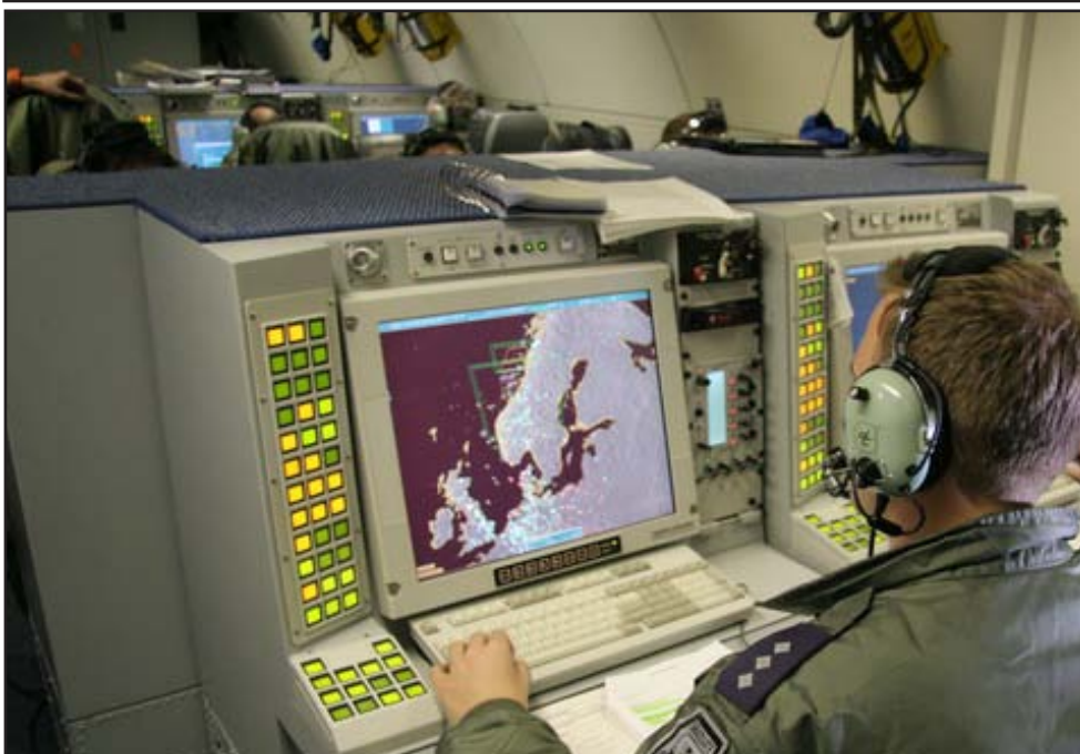
Radar Console inside a NATO Boeing E3-A AWACS Source: Metternich/NTA
